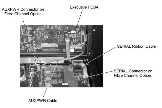
Figure 9-4 Detail of AUXPWR and SERIAL Connections in a Type A FCO
